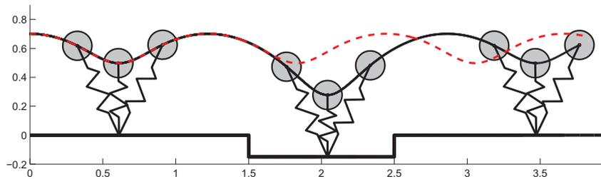
Fig. 3. CoM trajectory of the SLIP model adjusting the leg angle with constant leg length to have symmetric gait.<sup>4</sup>
