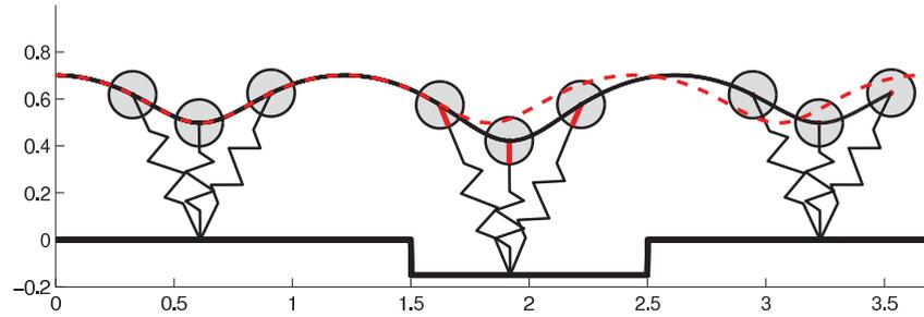
Fig. 6. The actuated SLIP model rapidly extends the leg and adjusts the leg angle concurrently. The red line on the leg at the drop gait is the increased leg length.
