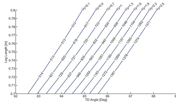
Fig. 4. Leg length vs leg angle for equilibrium gait policy with different vertical velocities. Numbers on the lines show the peak leg force [N] during the stance phase at that point. The peak forces are nearly constant along each curve.
