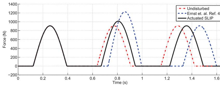
Fig. 7. Leg force profiles show the peak force increases only 11% if the leg is rapidly extended. This increase is due to the physical limitations of the motor like motor inertia. Without leg extension, increase in leg force would be 33%.
