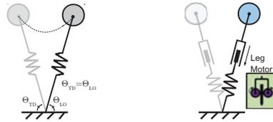
Fig. 2. **Left:** The passive SLIP model **Right:** The actuated SLIP model.
