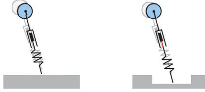
Fig. 5. **Left:** The leg actuator does not work on even ground (no leg extension, only leg angle adjustment during the flight phase) **Right:** The leg actuator extends the leg, the leg angle is adjusted concurrently based on the current leg length.
