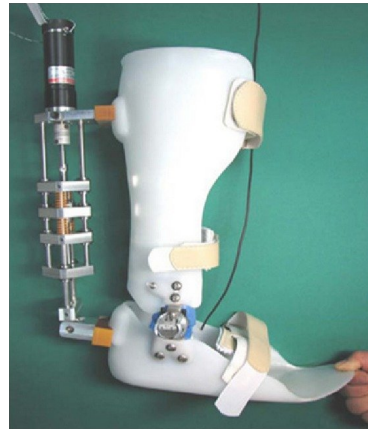
(b) A series elastic actuator powered ankle orthosis (Alam et al. 2014)
